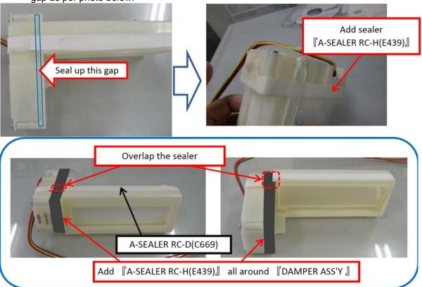
4) Add sealer RC-B part number PSEL-E465CBZZ on the slot of C-PART RF assy. Replace sealer RC-B part number PSEL-C563CBZZ with new thicker sealer as per photo below:
