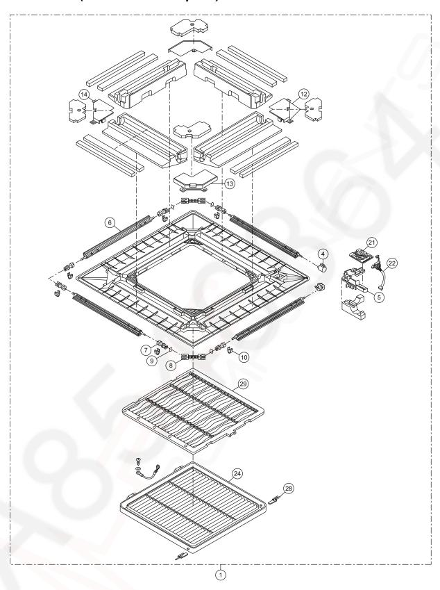
The above exploded view is for the purpose of parts disassembly and replacement. The non-numbered parts are not kept as standard service parts.
